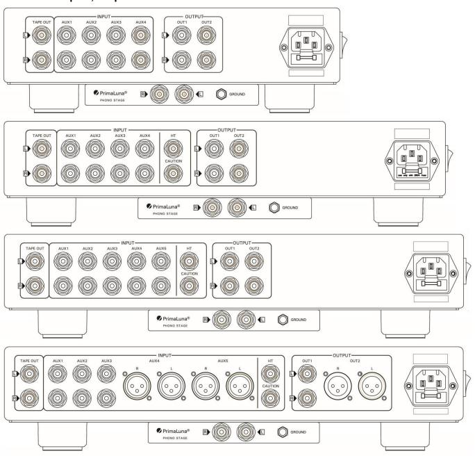
At the rear panel, you will find your inputs, eventually the HT Pass-Thru, Tape Out and preamp outputs.
