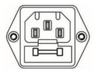
**Mains Fuse:** The mains fuse is located on the rear of the preamplifier, just below the power cord socket (see picture on the left). The fuse rating is 1 x Littelfuse 213 Series 1A Slow Blow 5 x 20mm fuse for 100-125VAC and Littelfuse 213 Series 0.5A Slow Blow 5 x 20mm fuse for 200-250VAC. Always replace with the same type and value fuse! The fuse holder can be opened using a small slotted flat blade screwdriver.
